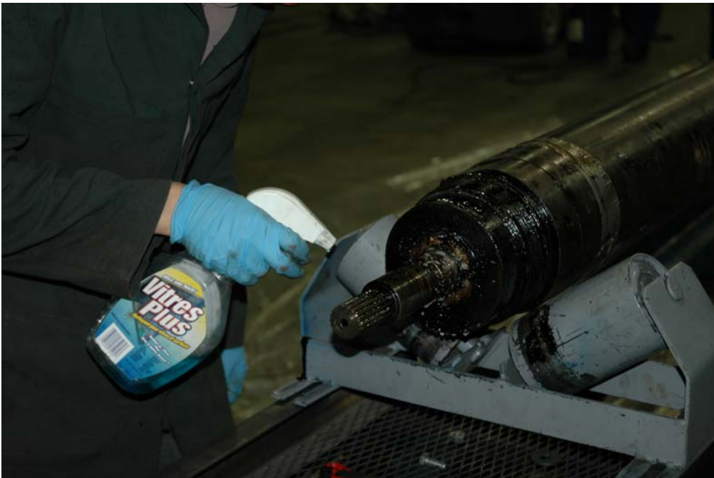
Bottom Mechanical seal tested for leaks under pressure.
