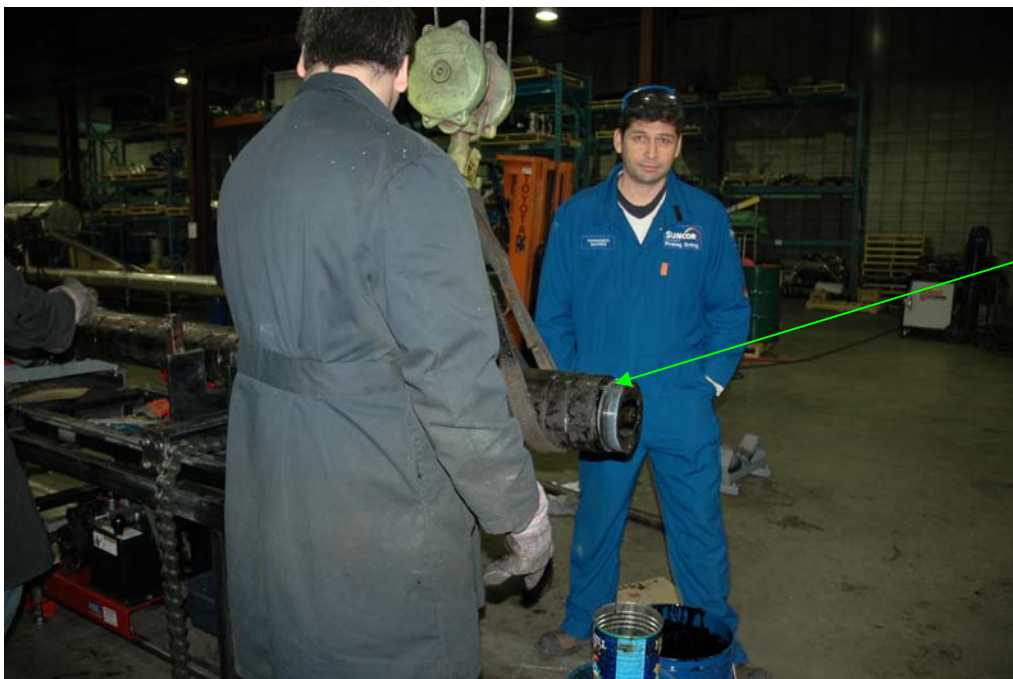
All thread connections between faces showed no leaks. Original thread dope is shown.
