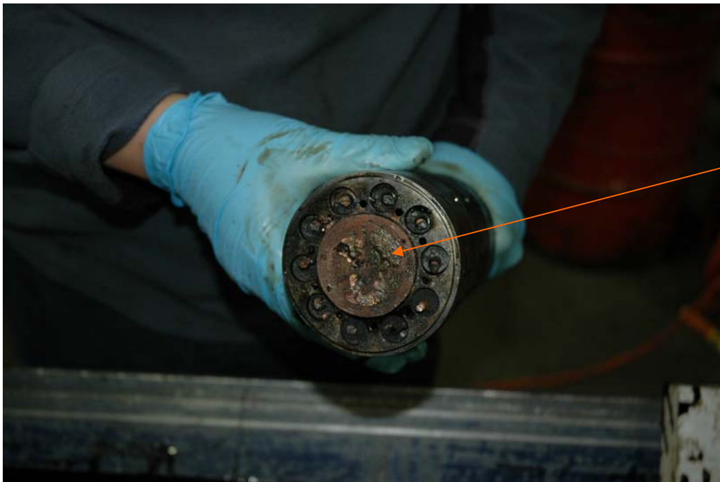
Main shaft Sheared with thrust bearings damaged
