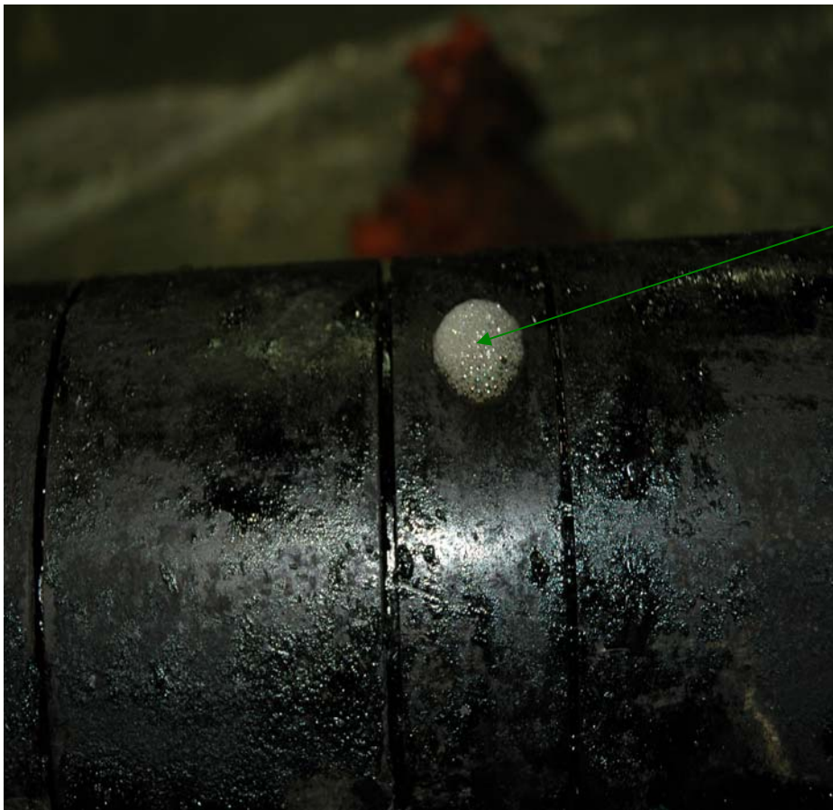
ORB pressure test on the thrust module. Showing Leaks on the ORB.
