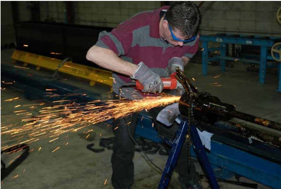
Cutting of metal pieces to remove main thrust bearings which are welded on due to high heat.
